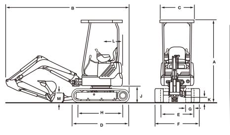
2350mm B: 3420mm C: 890mm D: 1560mm E: 990mm F: 1320mm G: 230mm H: 1210mm J: 445mm K: 175mm 640mm M: 250mm
